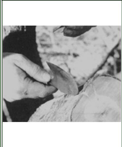
Figure 12. Knife with a half circle blade.
