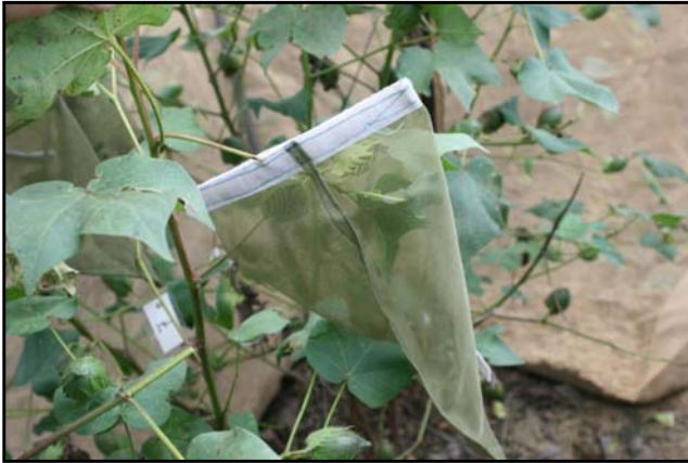
Small sleeve cage for confining stink bugs on cotton bolls.
